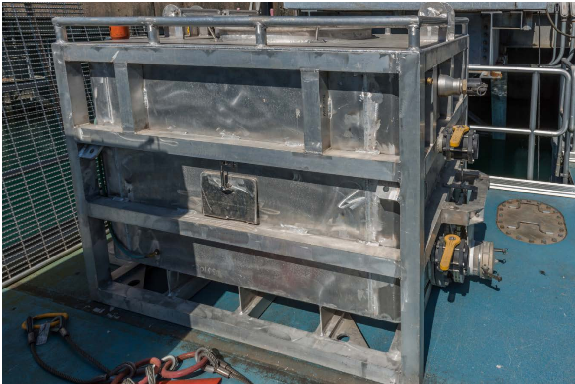
Figure 9. The water-filled transport tank for juvenile salmon. (Photo courtesy of Tony Grover)
