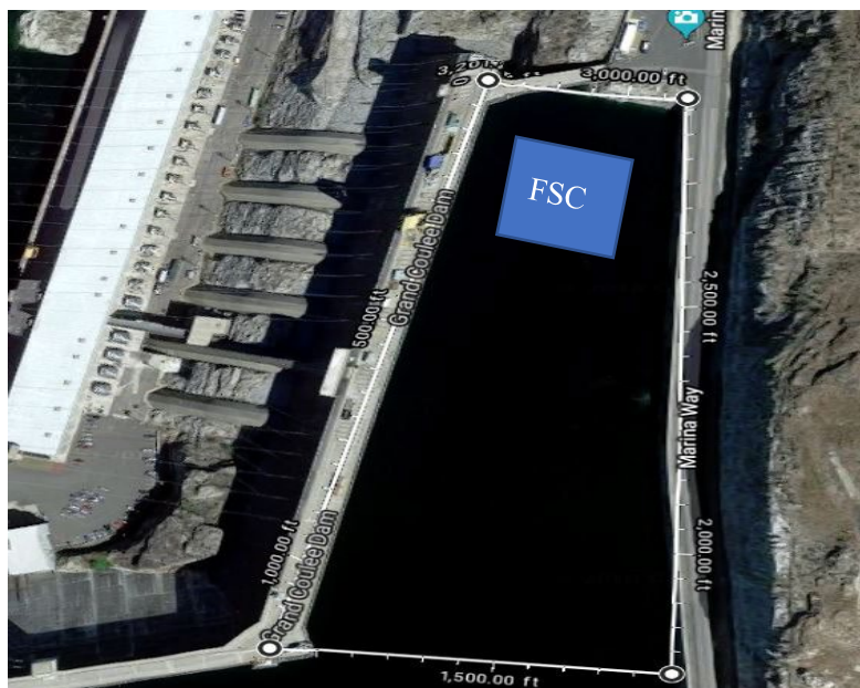
Figure 2. Image showing potential location for a floating surface collector (blue box) at Grand Coulee Dam. White line denotes powerhouse effective forebay area. Total effective forebay area is 11 acres.
