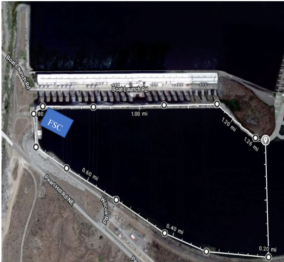
Figure 1. Image showing the potential location of a floating surface collector (blue box) at Chief Joseph Dam. White line denotes powerhouse effective forebay area. Total effective forebay area is 51 acres.
